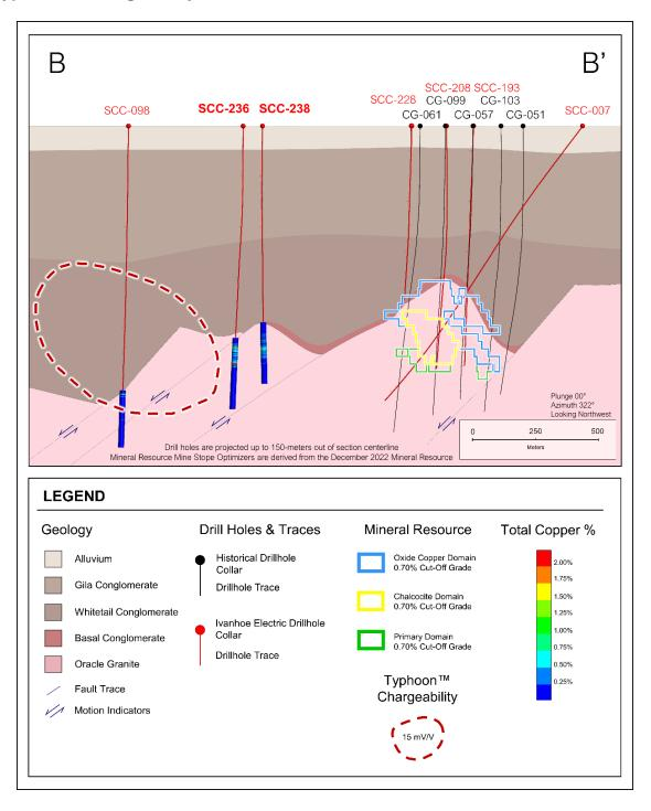
Exploration drilling in the Battle Butte Area at the Hog Heaven Project intersected a porphyry copper-gold-molybdenum system within a large, deep Typhoon™-identified anomaly
